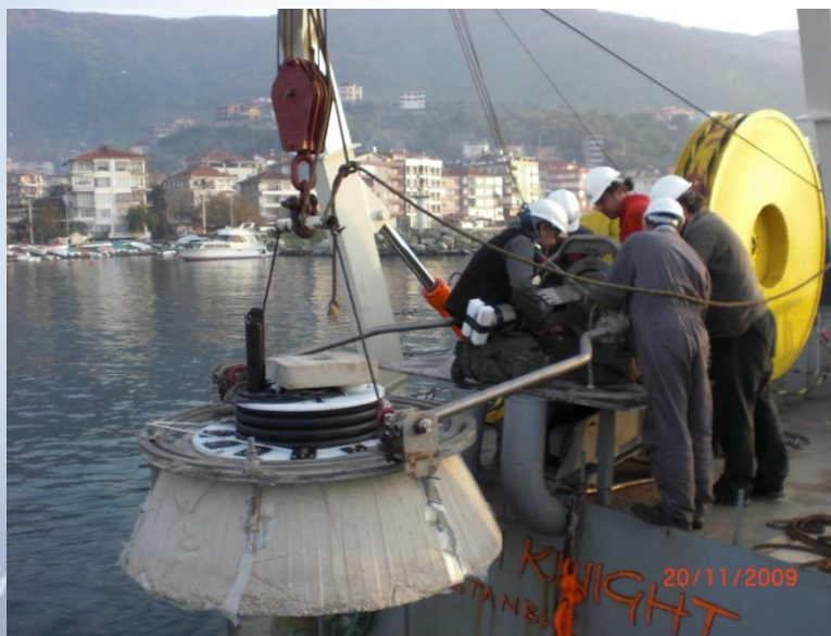
Installation of a seafloor station in the Sea of Marmara (KOERI)
