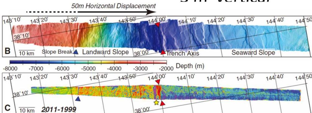
Repeated bathymetry sounding: ~ 50 m offset
